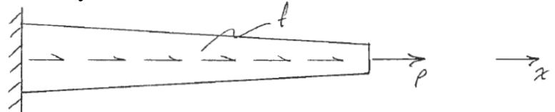
$$\Pi = U + V = \int_0^L \frac{F_N^2 dx}{2EA} - \int_0^L fu dx - Pu_{x=L} = \frac{1}{2} \int_0^L EA \left(\frac{du}{dx}\right)^2 dx - \int_0^L fu dx - Pu_{x=L}$$
