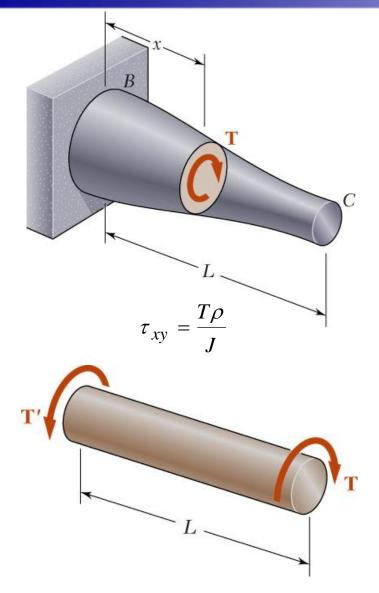
For a shaft subjected to a torsional load,
