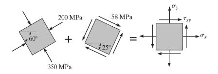
2. The state of stress at a point in a member is shown on the element. Determine the stress components acting on the inclined plane AB.
