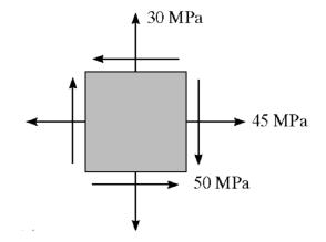
4. The stress at a point is shown on the element. Determine the principal stresses and the absolute maximum shear stress.
