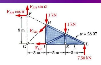
$$\tan \alpha = \frac{FG}{GL} = \frac{8 \text{ m}}{15 \text{ m}} = 0.5333 \qquad \alpha = 28.07^{\circ}$$
