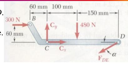
$\sum M_C = 0 = (F_{DE} \sin \alpha)(250 \text{ mm}) + (300 \text{ N})(60 \text{ mm}) + (480 \text{ N})(100 \text{ mm})$   $F_{DE} = -561 \text{ N}$  $F_{DE} = 561 \text{ N}$
