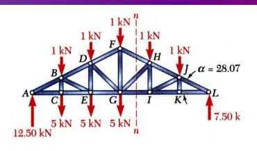
• Pass a section through members *FH*, *GH*, and *GI* and take the right-hand section as a free body.
