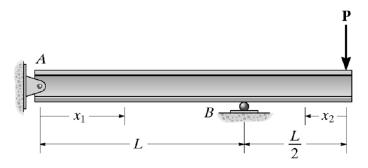
2. Determine the equations of the elastic curve for the shaft using the  $x_1$  and  $x_3$  coordinates. Specify the slope at A and the deflection at the center of the shaft. EI is constant. 【运用坐标  $x_1$ 和  $x_3$ 求图示梁的挠曲线,并求截面 A 的转角和梁中点处的挠度。设弯曲刚度 EI为 常数。】
