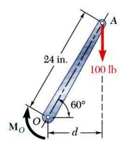
e) Although each of the forces in parts b), c), and d) produces the same moment as the 100 lb force, none are of the same magnitude and sense, or on the same line of action. None of the forces is equivalent to the 100 lb force.
