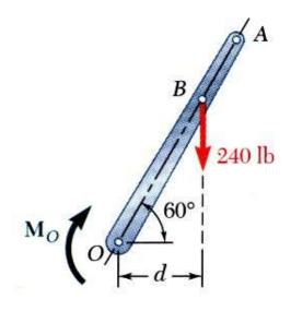
d) To determine the point of application of a 240 lb force to produce the same moment,
