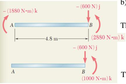
b) Find an equivalent force-couple system at *B* based on the force-couple system at *A*.
