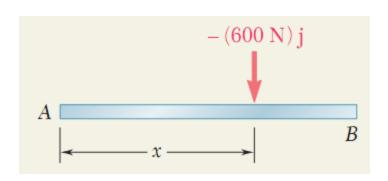
c) The resultant of the given system of forces is equal to R, and its point of application must be such that the moment of R about A is equal to  $M_A$
