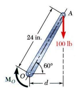
a) Moment about *O* is equal to the product of the force and the perpendicular distance between the line of action of the force and *O*. Since the force tends to rotate the lever clockwise, the moment vector is into the plane of the paper.
