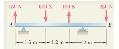
For the beam, reduce the system of forces shown to (a) an equivalent force-couple system at *A*, (b) an equivalent force couple system at *B*, and (c) a single force or resultant.
