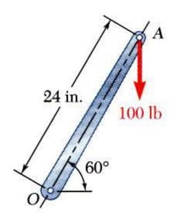
A 100-lb vertical force is applied to the end of a lever which is attached to a shaft at *O*.
