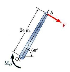
c) The smallest force *A* to produce the same moment occurs when the perpendicular distance is a maximum or when *F* is perpendicular to *OA*.
