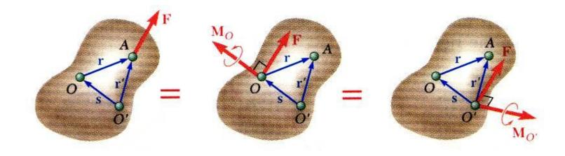
• Moving F from A to a different point O' requires the addition of a different couple vector  $M_{O'}$ .
