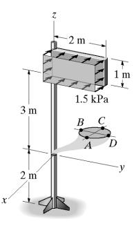
4. The solid rod is subjected the loading shown. Determine the state of stress at point *C*, and show the results on a differential volume element located at this point.
