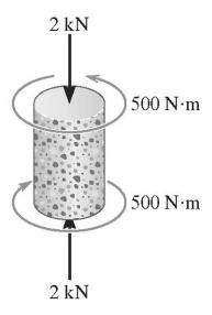
2. If a solid shaft having a diameter d is subjected to a torque T and moment M, show that by the maximum normal stress theory the maximum allowable principal stress is
