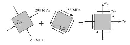
2. The state of stress at a point in a member is shown on the element. Determine the stress components acting on the inclined plane AB.
