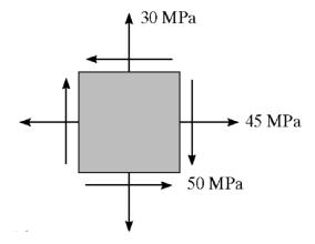
4. The stress at a point is shown on the element. Determine the principal stresses and the absolute maximum shear stress.
