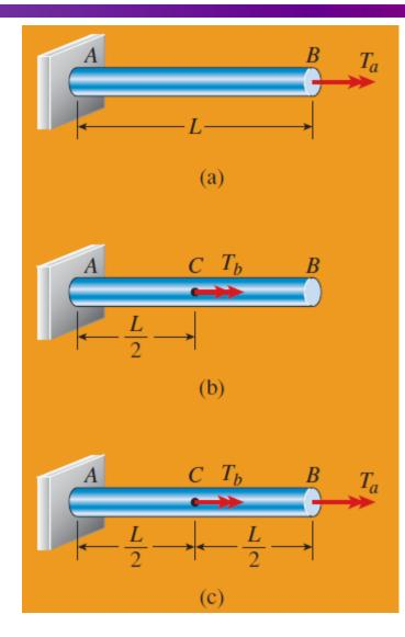
• A solid circular bar is fixed at one end and free at the other. Three different loading conditions are to be considered. For each case of loading, obtain a formula for the strain energy stored in the bar.
