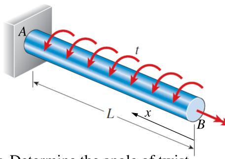
• Determine the angle of twist at end *A* of the shaft.
