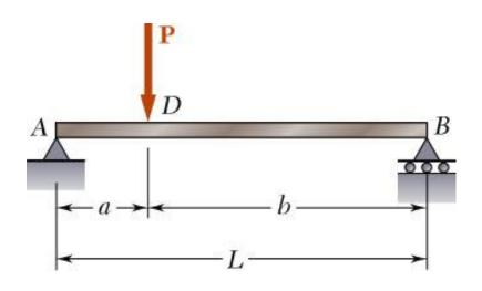
Taking into account only the normal stresses due to bending, determine the vertical displacement at cross-section D of the beam for the loading shown.
