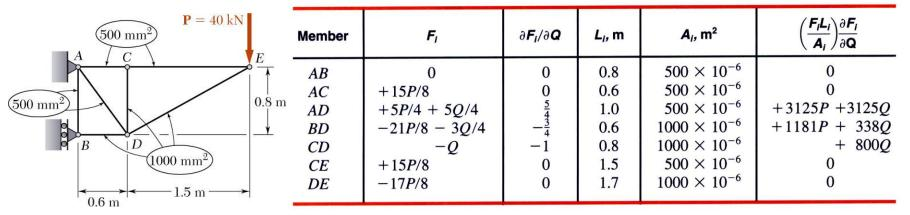
• Combine with the results of previous example to evaluate the derivative with respect to Q of the strain energy of the truss due to the loads P and Q.
