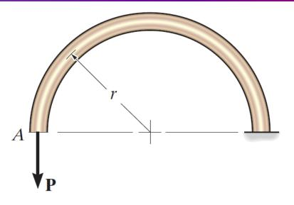
• Determine the vertical displacement at *A*. Only consider the strain energy due to bending. Assume constant flexural rigidity *EI*.
