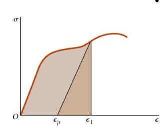
• To eliminate the effects of size, evaluate the strainenergy per unit volume,
