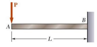
• For an end-loaded cantilever beam, M = -Px
