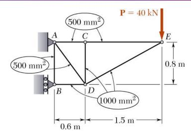
Members of the truss shown consist of sections of aluminum pipe with the cross-sectional areas indicated. Using E = 73 GPa, determine the vertical deflection of the joint *C* caused by the load *P*. Solution:
