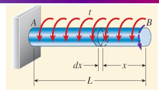
• Determine the angle of twist at cross-section *B* of the shaft.
