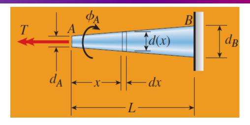
• Determine the angle of twist at end *A* of the shaft by equating the strain energy to the work done by the load.
